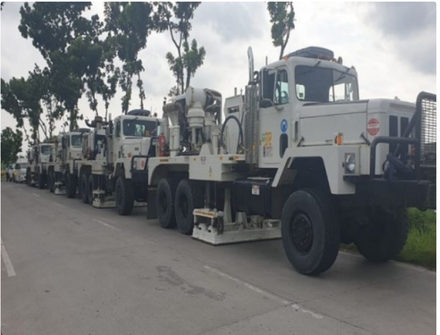
Survey Seismik 2D Vibroseis/foto: dok Pertamina
